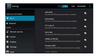
❖ Wi-Fi: Turn on or turn off WLAN function
